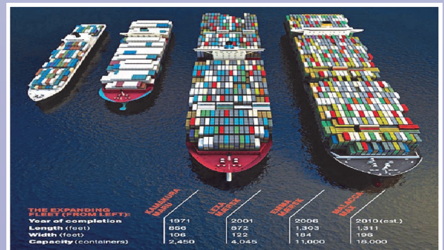
This illustration shows the mix of vessels that will be used in the Port of the Americas and the enormous size of post-Panamax vessels. From left, a feeder vessel, a Panamax vessel, a post-Panamax vessel that is currently in use, and at the far right, the latest and largest post-Panamax vessel that will be in use in 2010.
